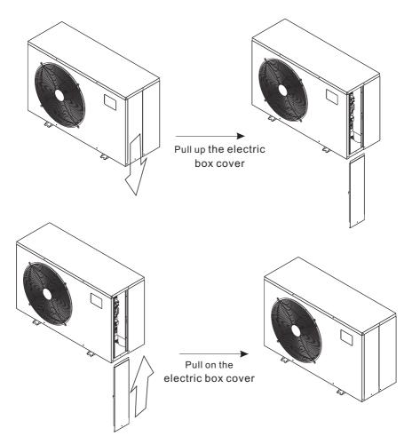
Attention: 1. Please be careful when handle with the electric box cover in case of damage; 2. During installation to buckle matched with the clamping groove of the electric box cover, so that it can cover the electric box cover.
