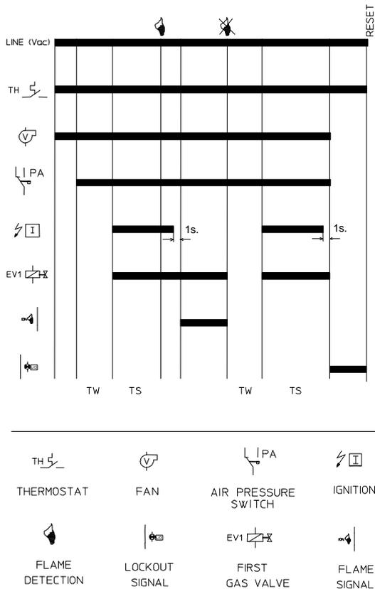
After checking the air pressure switch opening, the FCM unit starts the fume extractor, and after a check of the air flow, the ignition stage begins by counting the prepurge and safety times, as shown in the diagram below.
