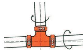
6. Coupling keys engage the full circumference of the grooves and provide significant pressure and end load restraint against pipe movement from internal and external forces.
