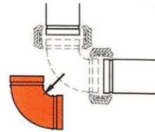
5. Couplings are non-directional and pipe can be rotated 360° during installation.
