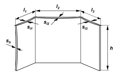
Fig. 7.1: Angular bent ROBAX® panels
