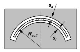
Contour slot gauge geometry for round bent ROBAX® panels Fig. 6.2:
