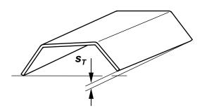
Overall torsion of an angular bent ROBAX® panel Fig. 7.2:
