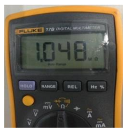
Figure 4-4.4: Measuring resistances among compressor terminals
