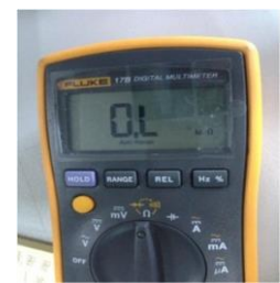
Figure 4-4.5: Measuring resistances between compressor terminals and ground
