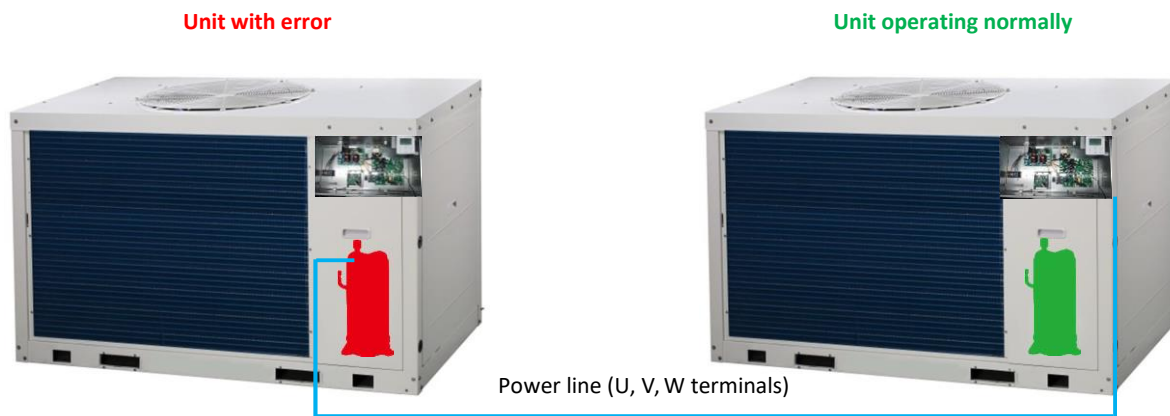
Figure 4-4.10: Connecting compressor to an error-free unit
