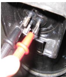
Figure 4-4.4: Measuring resistances among compressor terminals
