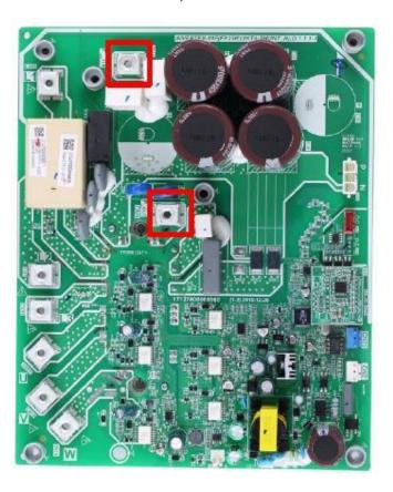
2. The normal resistances of the inverter compressor are 0.7-1.5Ω among U V W and infinite between each of U V W and ground. If any of the resistances differ from these specifications, the compressor has malfunctioned.
