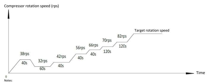
1. Once the first, 40-second stage of the program is complete, the program proceeds to the subsequent stages in a step-by-step fashion and exits when the target rotation speed has been reached.
