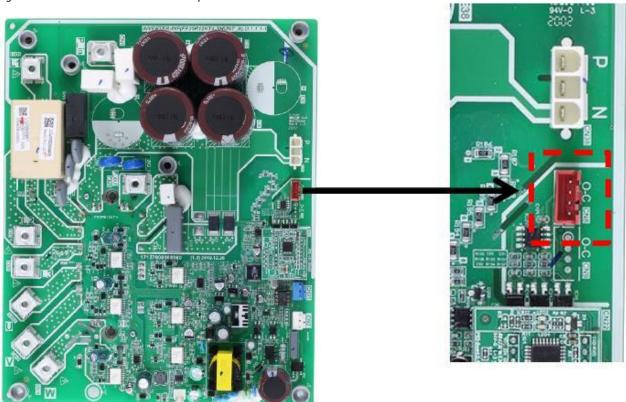
When replacing an inverter module, a layer of thermally conductive silica gel should be painted on the IPM module (on the reverse side of the inverter module PCB). Refer to Figure 4-4.2.
