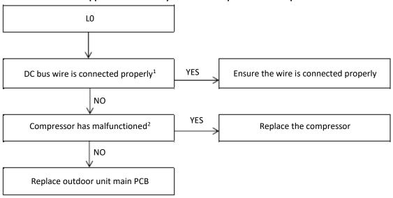
1. The DC bus wire must run from terminal N on the inverter module, through the current sensor (indicated by the arrow on the current sensor) and end at terminal N on the capacitor. Refer to Figure 4-4.7.
