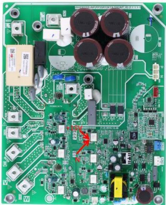
3. Check the +15V circuit according to the corresponding wiring diagram. If the output power supply of the inverter module in IC4/5/6PIN12 is not +15V, the inverter module is faulty. If the output power supply of the inverter module is +15V, the main PCB is faulty.
