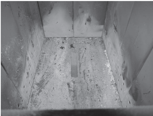
Pic. 6 Correctly cleaned feeding chamber
