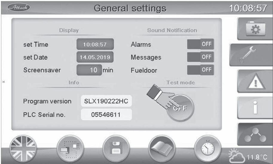
Pic. 24 Finishing of the boiler's test mode
