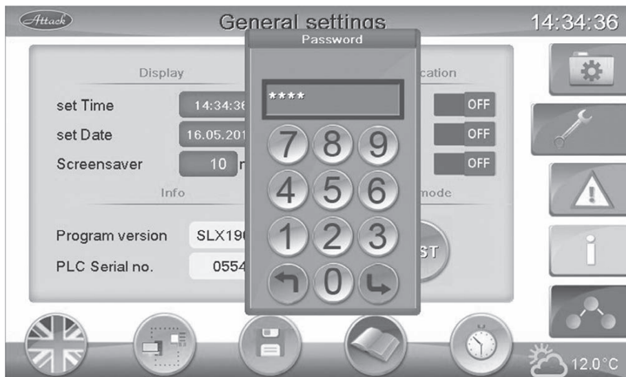
Pic. 53 Access to advanced parameters
