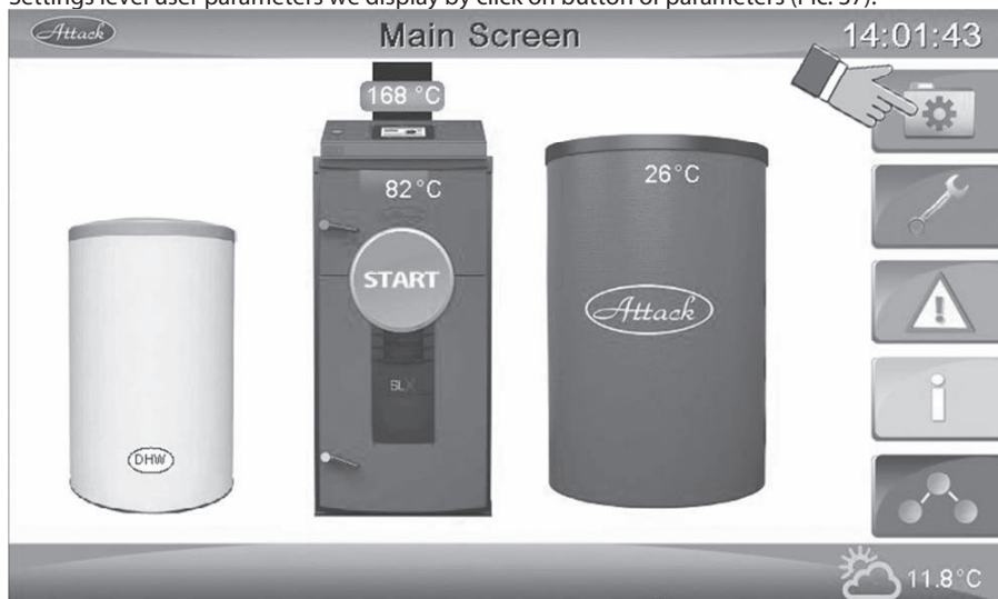
Pic. 37 Clicking on displaying of parameters
