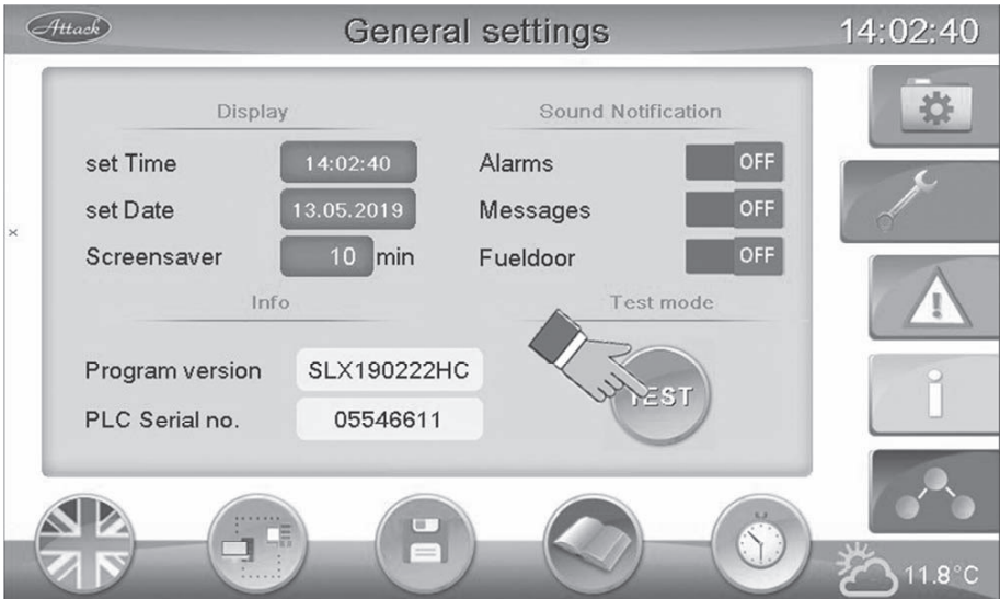
Pic. 20 Entry into TESTMODE
