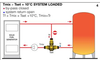
Tmix = Mixed water temperature of generator return Tr = System return temperature
