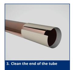
• Clean the end of the tube, ensuring that it is round and undamaged.
