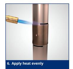
• Apply heat, moving the flame to ensure that parent metals and fitting are evenly heated.
