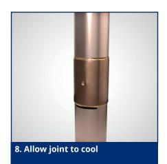
• Once brazed, discontinue heating. During cooling, **do not** move or twist the components.
