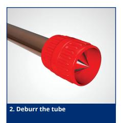
• Deburr the tube internally and externally.
