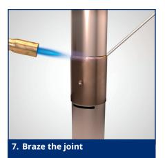
• Touch a brazing rod, strip or wire to the joint mouth and melt in the flame.
