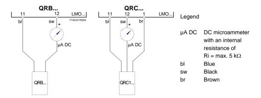
As an alternative to detector current measurement, the diagnostic tool OCI400 / ACS400 can be used. In that case, the DC microammeter is not required.
