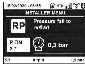
Figure 18 Setting the restart pressure
