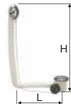
Coloan scurgere cad cu dop i lan Universal waste pipe for bathtub with plug and chain
