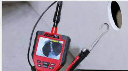
Cavity wall inspection, locating and capturing
