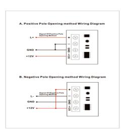
A. if you want to connect the positive side to open the lock :please connect the contact "L -" and "GND" with A short wires, otherwise it cannot control the lock;(Please check the wiring diagram --A)
