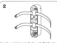
Use the metal strap to fix the unit. Tightly strap the unit on a gutter.
