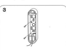
After BACK BOX is installed, magnetic contact should be connected with tamper terminal through the cable hole.
