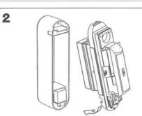
After cabling between transmitter and the unit can be fixed with 2 screws. Hook the unit onto the BACK BOX fasten turn 2 lock screws on the unit below.
