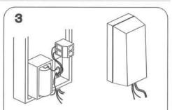
Use enclosed alarm cable to connect with alarm imput terminal and draw cables out and close the cover.
