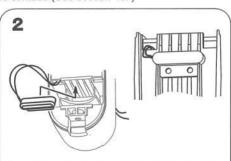
Magnetic contact with cable should be fixed on the bottom part of the BACK BOX.
