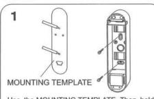
Use the MOUNTING TEMPLATE. Then hold the template against the mounting surface, when BX-80NR is to be mounted. Mark the position of the mounting hole then discard template. Then fasten the unit on the marked position.
