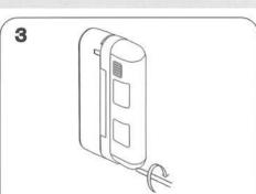
Put the cover on and conduct walk test. After completed turn the lock screw on the cover.
