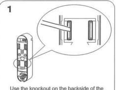
Use the knockout on the backside of the BACK BOX.
