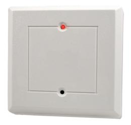
The DS1102i Detector Series uses microprocessor-based sound analysis technology (SAT) to listen for the specific frequencies associated with breaking glass. The DS1102i and DS1102i-CHI can be used to detect breakage of plate, tempered, laminated and wired glass types. A built-in environmental test feature alerts the installer to false alarm hazards in harsh environments. The square detectors mount on ceilings or walls.
