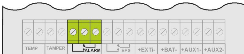
Fig. 8. Technical output ALARM.
