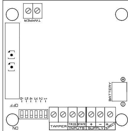
**TAMPER Clamps:** N.C. Antiopening and Tearing Off Contact
