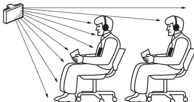
Figure 4.9: Infrared signal blocked by a person in front of the participant
