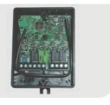
Outdoor two-channel and four-channel receivers, with cable connection, 12-24 Vac Vdc power supply, including integrated radio signal decoding. Suitable for fixing on DIN rail.
