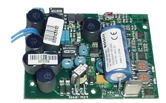
The board monitors the integrity of a loudspeaker. It works together with the LBB 4440/00 Supervision Control Board. The speaker status is communicated to the LBB 4440/00 via the existing loudspeaker cable.
