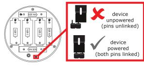
Once powered, reassemble the device.
