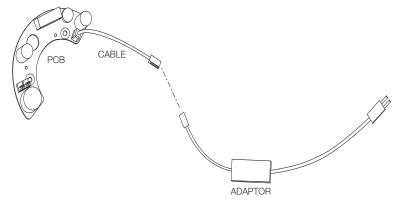
6. After inserting the external camera cable to the housing, connect to the corresponding jack on the adaptor.
