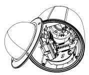
7. Please install the camera onto the housing. Please confirm that the adaptor hook is properly fixed on the camera.
