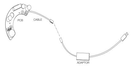
After inserting the external camera cable into the housing, connect it to the corresponding jack on the adaptor.
