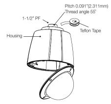
4. Install on the pipe by turning the housing in a clockwise direction, referring to the figure below.
