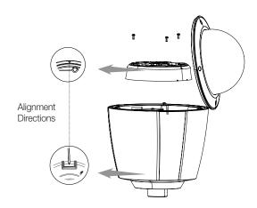
2. Please pull out the external cables to the outside through the inner part of "pipe or mount". Please apply the Teflon taping around the screw part of the "housing."
