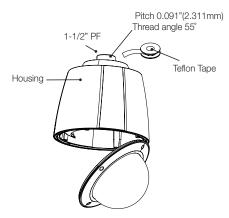
3. Install onto the pipe by turning the housing in a clockwise direction while referring to the figure below.
