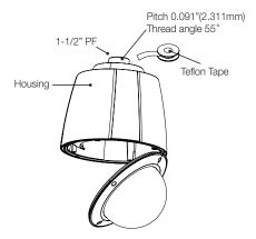
4. Install onto the pipe by turning the housing in a clockwise direction while referring to the figure below.
