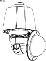
8. After confirming that the unit has been installed properly, attach the housing cover and tighten it firmly using 4 screws.
