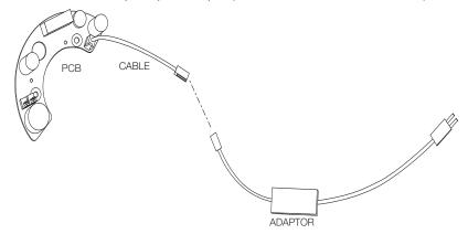
After connecting the camera adaptor and inner cable while referring to the installation manual, install the camera onto the housing and check if the adaptor hook is fastened properly onto the camera.
