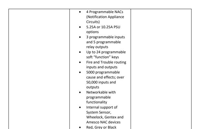
There are many configurations available on the Taktis relating to the number of zone indications, internal power supply, number of apertures, printer options etc.
