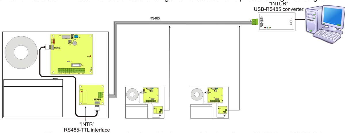
Fig. 14. RS485 communication with the use of the interfaces: "INTR" and "INTUR".
