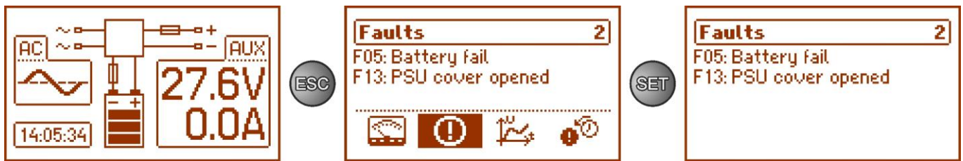
Fig. 10. LCD screen – current failures of the PSU.
