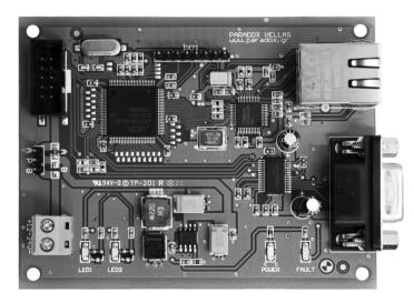
SRTCP-IP module connects directly with SmartX panel's main board ("TO TCP/IP BOARD" connector). SRTCP-IP gives the ability to program and control the SmartX fire alarm panel through the ethernet / internet (TCP/IP) in real time with the use of the specially designed SmartView software.
