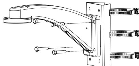
2. Install the PTZ pole mount adapter to a pole using the three hose clamps.
