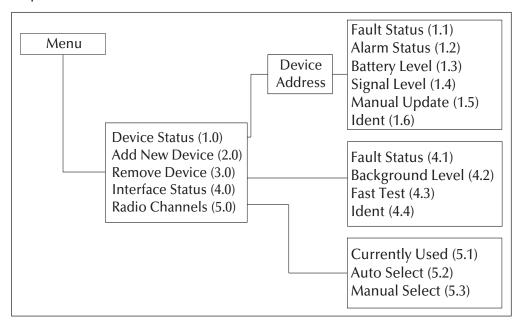
A rotary select switch is used for scrolling through the menu and selecting an option. Turn the select switch clockwise to scroll down the menu. Turn the switch anti-clockwise to scroll back up the menu. Press the select switch once to select an option.
