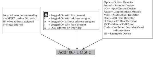
Note: Combined sounder visual indicator base shows two addresses, first address in the detector followed by the sounder visual indicator as shown below.
